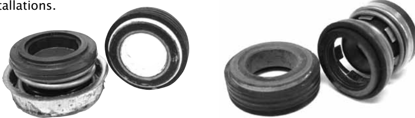
PTFE or Silicone Based Lubricants Destroy Seals
