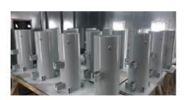
TransArmour provides engineered innovative coatings by utilizing the very latest technology to solve corrosion issues on the grid. Our advanced coating formula is designed for application on utility equipment as an alternative to stainless steel in corrosive environments. We also offer new and rebuilt transformers utilizing TransArmour coating solutions.
