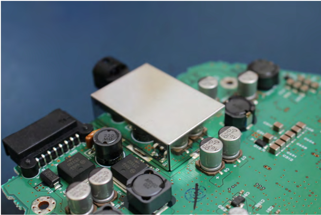
Figure 6. RF shielding soldered to PCB.
