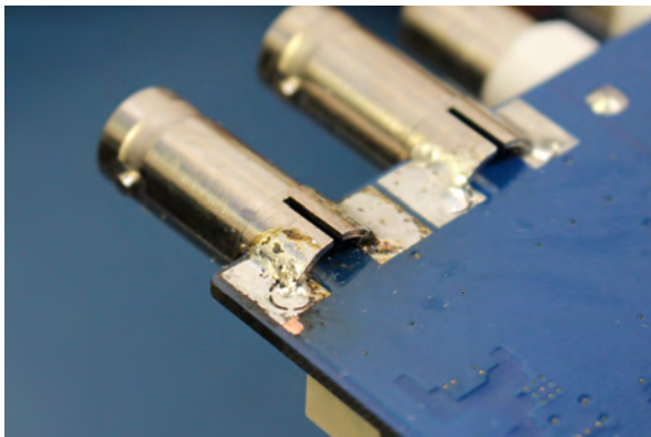
Figure 4. Burnt solder joint due to too much heat while soldering
