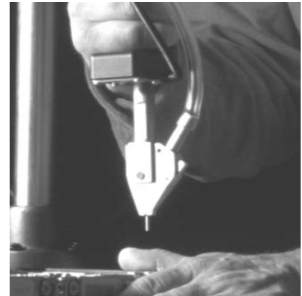
Narrow pointed jaws provide maximum screw visibility
