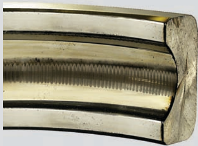
Bearing fluting, "washboard" pattern on bearing race
