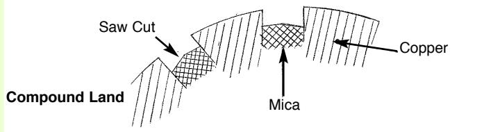
After a commutator has been undercut, it should be very carefully inspected to assure that all copper particles have been removed, that the bars have been carefully chamfered, and that all sharp edges and burrs have been eliminated. Then each slot should be individually checked and reworked as necessary to remove any traces of fin or side mica.
