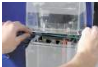
Select job, insert wire or cable.
